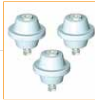
M8 Set of 3 Ø89 x 76 Polyfiber Base Insulators supplied with M7 pedestal base with 3 x 15 mm slots on 200 mm - 254 mm PCD
