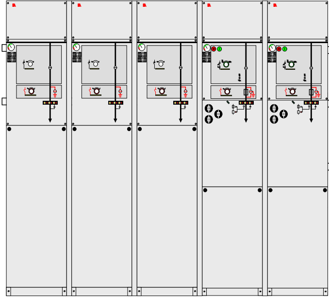
SafePlus 36 with a fully modular design
